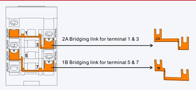
\* Warning: Verify that all connections (including bridging link connections) are suitable for the rated current, prepared to ensure only conductive parts are clamped and tightened to the manufacturers required torque before energization.
